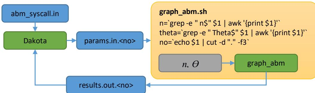
Figure 10: Coupling the demonstration application to Dakota.
