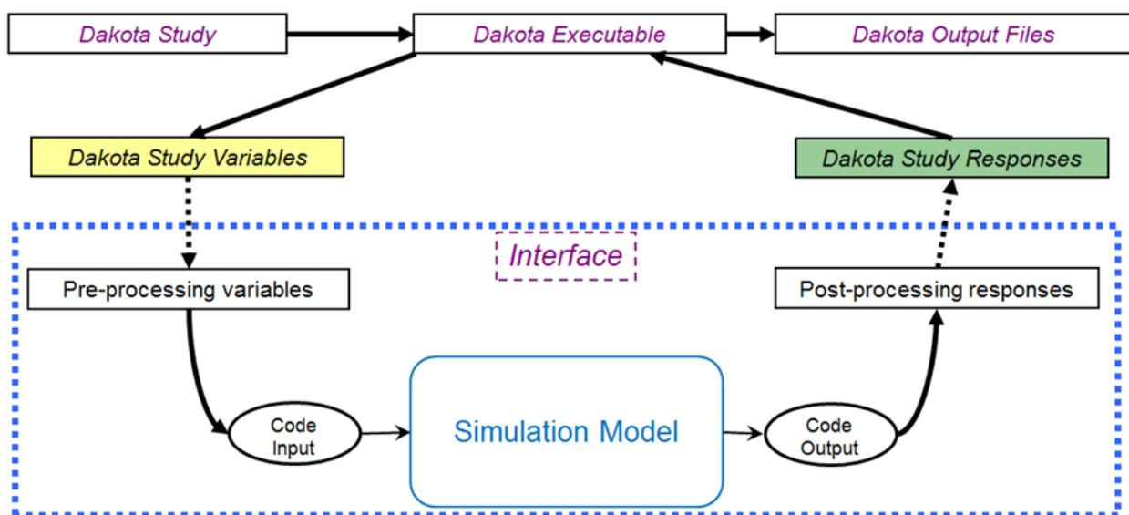
**Figure 8: Dakota flowchart for running external simulation models. (Adams, 2017)**
